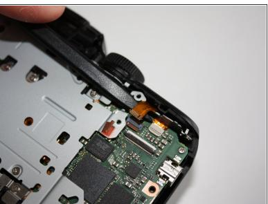
Gently flip up the flex ribbon lock and remove the flex ribbon.
