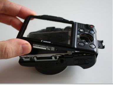
• Once all screws are removed, open up the back case with a plastic opener from the left side.
