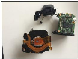
• Gently flip up the flex ribbon lock and remove the flex ribbon.
