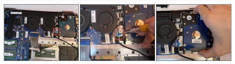
• Disconnect the clip attaching the hard drive cable to the motherboard.
