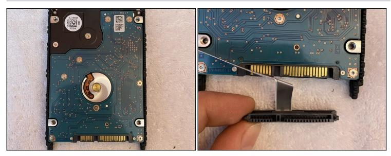
• Reattach the side brackets and the hard drive connector.
