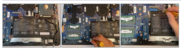
• Remove the four 2x5 screws using the Phillips screwdriver.
