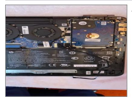
• Slide the battery out of its space to remove it from the computer.
