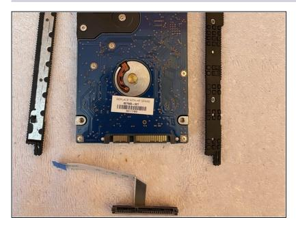
• Disassemble the hard drive by removing the connector and the side brackets.
