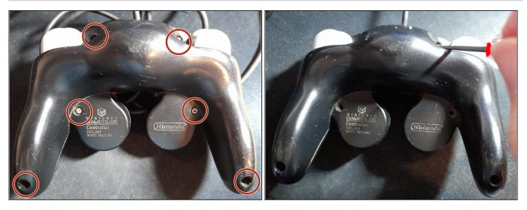
Using the Tri-Wing, remove the six 9.2mm Tri-wing Y0 screws at the back of the controller
