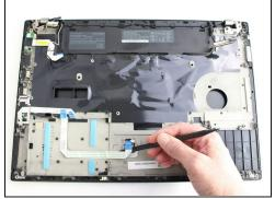
Using the black nylon spudger, remove the ribbon cable connected to the trackpad.
