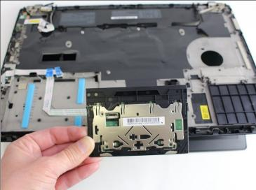
• Lift the chassis up and the trackpad will fall out.
