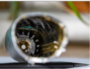
This just shows the hooks alongside the sledge holding the parts as well as the rails it slides on inside the frame.
