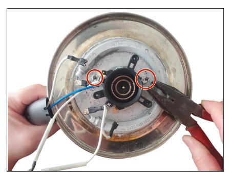
Use combination pliers to reinstall the nuts holding down the temperature controller.
