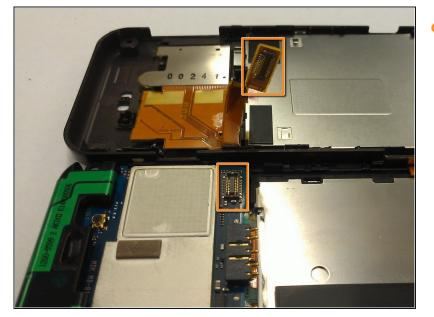
• With both insides of the phone exposed, gently detach the ribbon cable connecting the two inner sides. You can now separate the two sides of the phone.
