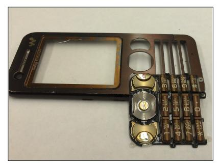
• Separate the front and back panels that were pryed open with the plastic opening tool.
