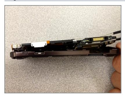
• Now that the faceplate is off, use <u>tweezers</u> to separate the backplate from the inner manifold.
