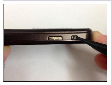
• Flick the two lock tabs into the unlocked positions by pushing each button forward.
