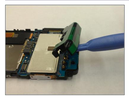
The motherboard is located on the side with the green and black bumper on the bottom. Use the plastic opening tool to pry the bumper off.
