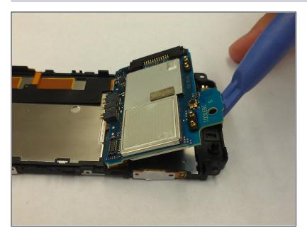
• To remove the motherboard, apply upwards pressure on the bottom green tab.
