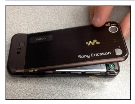
• Pop the back cover up using the groove on the top of the phone.
