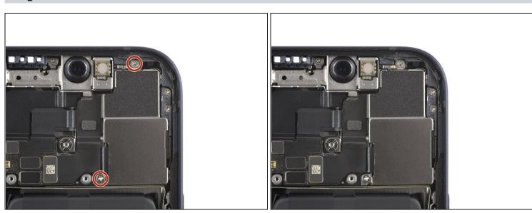
Remove the two 1.6 mm-long Phillips #000 screws.
