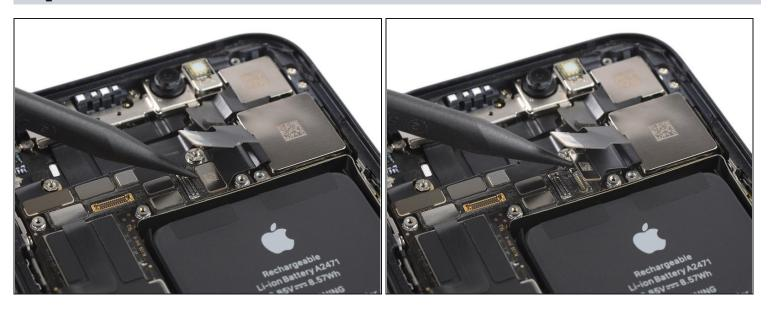
• Use a spudger to disconnect the wide camera flex cable by prying it straight up from its socket.
