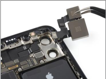
• Use a pair of tweezers to remove the camera module.
