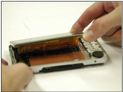
• Use a spudger to separate the metal tabs that hold the screen in place on the right side.
