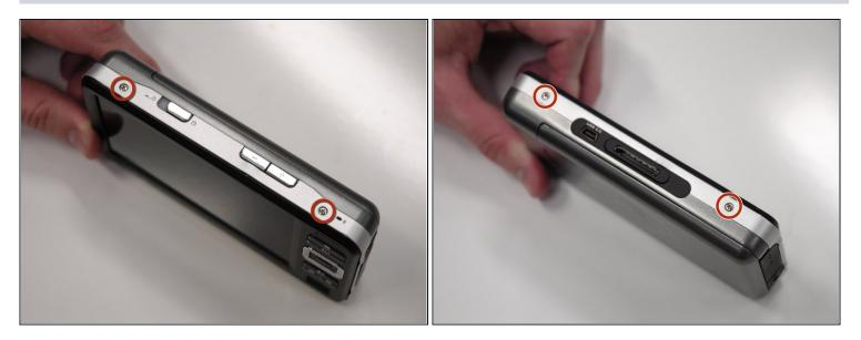
Remove the two screws (2.5 mm) on the top and bottom of the device using a Phillips #0 screwdriver.
