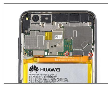
Use a Phillips #00 screwdriver to remove the two 2.9 mm-long screws securing the battery connector shield.
