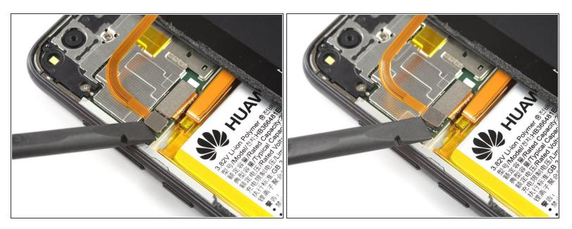
• Use a spudger to pry up and disconnect the fingerprint sensor cable.
