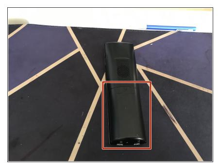
Remove the back cover by sliding it off.
