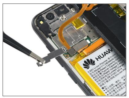
• Use a pair of <u>tweezers</u> to remove the metal shield.
