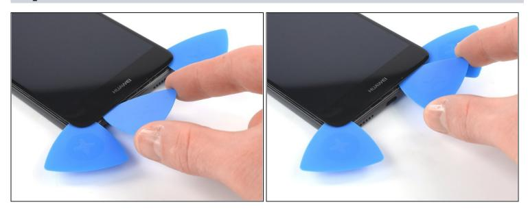
• Insert a fifth opening pick under the bottom left corner and slide it to the bottom right corner to cut the remaining adhesive.
