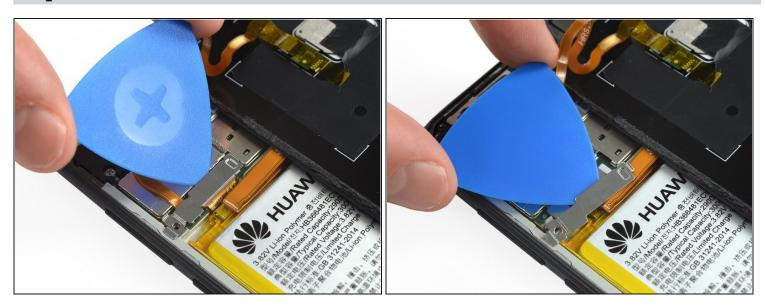
• Use the tip of an opening pick to pry up and loosen the metal shield.
