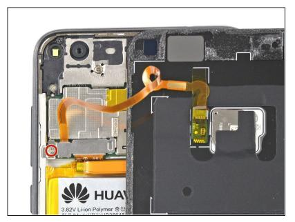
Use a Phillips #00 screwdriver to remove the 2.9 mm screw.
