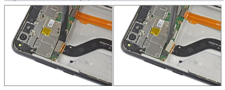
• Use a spudger to disconnect the display flex cable from the motherboard.
