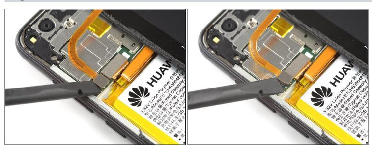
• Use a spudger to pry up and disconnect the fingerprint sensor cable.
