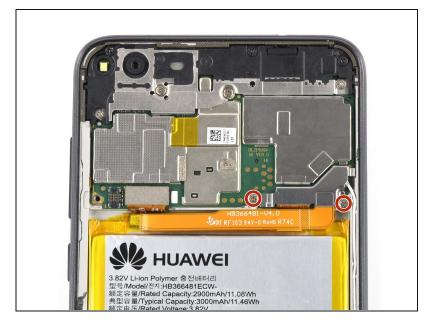
Use a Phillips #00 screwdriver to remove the two 2.9 mm-long screws securing the battery connector shield.
