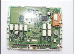
The board is exposed! Now simply push back the plastic tabs connecting the board and disconnect the cables
