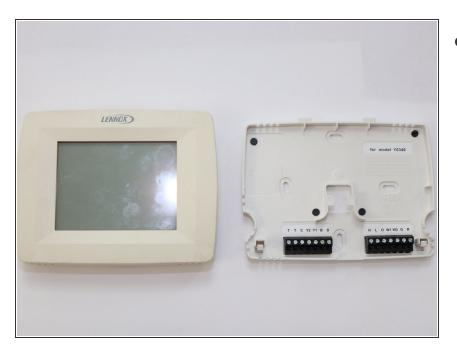
Pushing in at the bottom of the thermostat, pull down and remove the thermostat from the wall. Note: the circuit breaker for the HVAC system MUST be off. Use caution when handling electrical wires.
