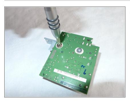
Remove both screws holding the retaining plate with the logic board.
