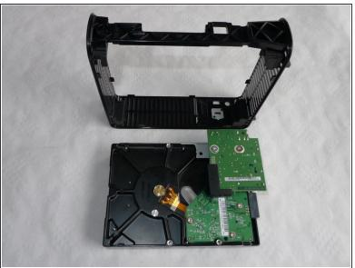
Slide out the hard drive as shown in the picture
