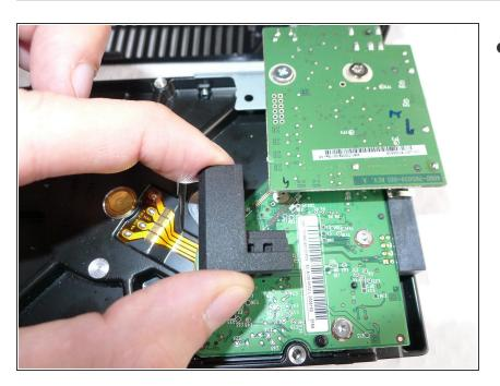
Remove the rubber piece from the SATA/USB bridge logic board.
