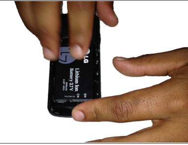
Remove the battery from the compartment to reveal the SIM card.
