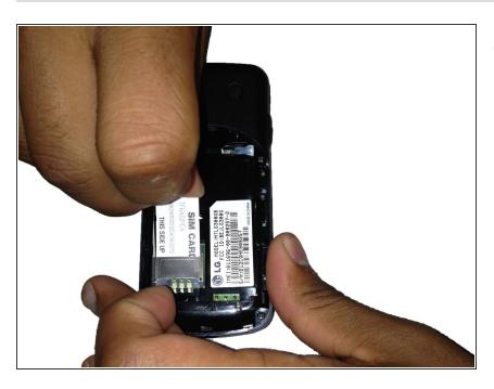
Remove the SIM card by pushing down on the top and slide it out from under the metal band upwards.
