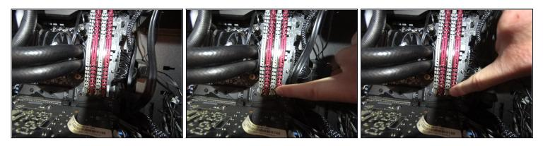
• If any of the clips did not properly lock back in place, apply pressure on the side of the RAM stick with the disengaged lock.
