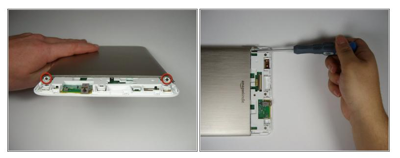
Use a Phillips #00 screwdriver to remove the two 4 mm screws from the metal casing.
