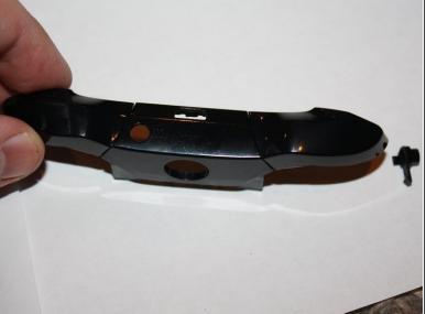
• Using your hands or a prying tool, gently remove the top bumper strip from the top of the controller.
