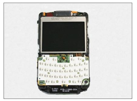
After disassembling the outer casing, the phone should be stripped as shown.
