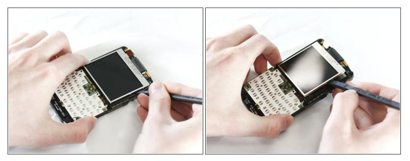
• Using the prying tool, lever up the old screen as shown.
