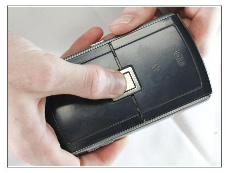
Remove the battery cover by applying pressure and sliding down the silver square on the back of the phone.
