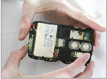
Unhook both sides of the white wire from the motherboard using the plastic opening tool from before
