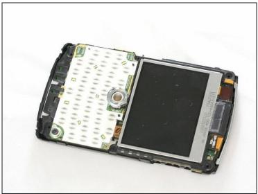
Remove the bottom casing clip, it will easily unsnap when pulled
