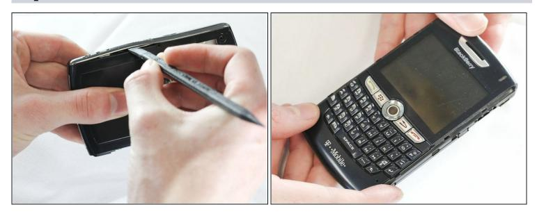
• Use a nylon spudger to carefully remove the two side bars of plastic.
