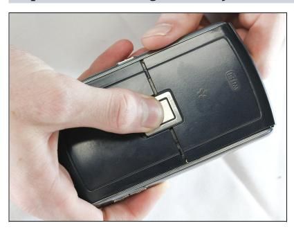
Remove the battery cover by applying pressure and sliding down the silver square on the back of the phone.
