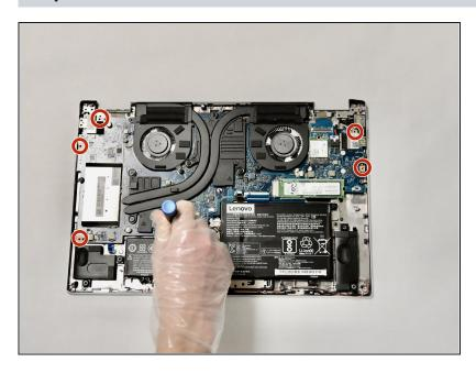
Using the Phillips #000 screwdriver, remove the five screws.
