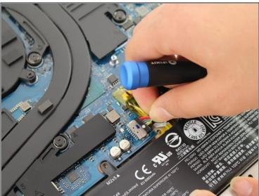
Pull firmly on the battery connector to disconnect it.
