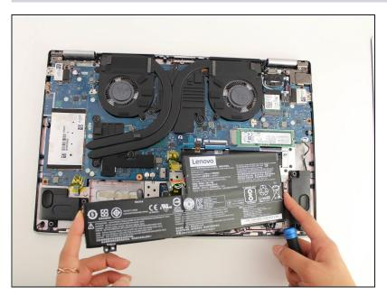
• Lift the battery out of the case to remove it.
