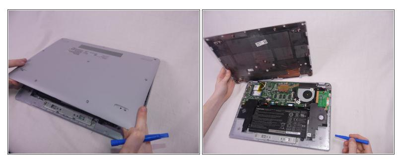
Remove the back cover by gently lifting up on one side of the device.
