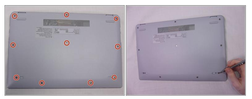
Remove the 10 7.1 mm screws using Phillips #1 screwdriver.
