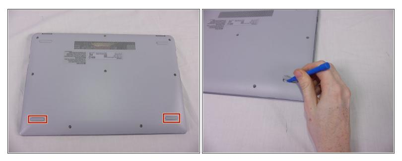
Remove the 2 rubber foot pads from the bottom (opposite the hinge) with the small Plastic Opening tool.
