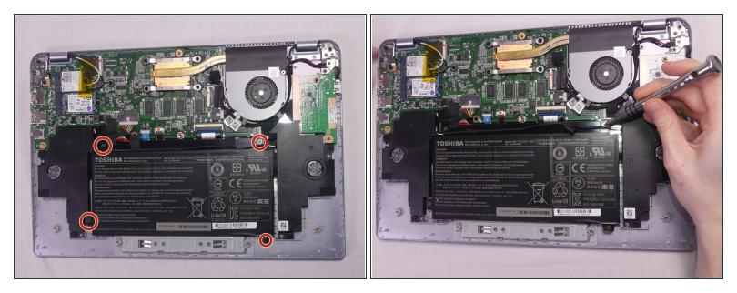
• Remove the 4 Phillips 3.2 mm screws holding the battery in place, with the Phillips #1 screwdriver.
