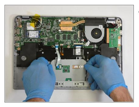
• Slide the trackpad up and out to remove the part.
