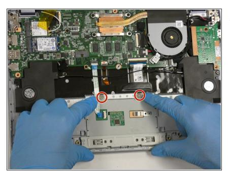
Using a Phillips #1 screwdriver, remove the two screws located at the top of the trackpad.
