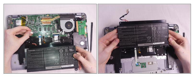
Remove the battery by gently pulling on the bottom corners.
