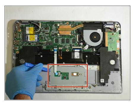
• Using an opening tool, gently lift up the edge of the trackpad.
