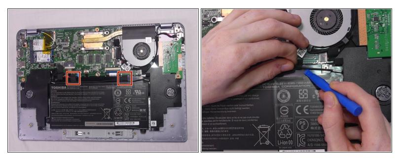
• Remove the tape holding the speaker wire to the battery on both sides using a small opening tool.
