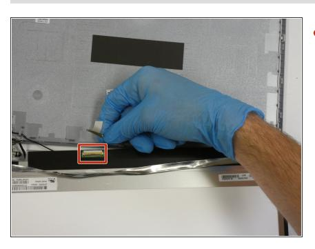
Carefully remove the ribbon the display and remove the display from the Chromebook.
