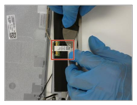
Using the Jimmy, remove the sticker holding the wire to this display.
