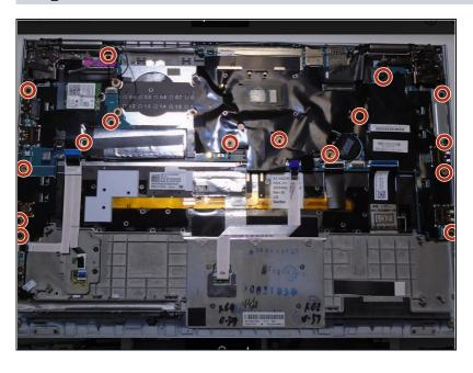
Using a Phillips #0 screwdriver, remove all 16 of the 6 mm screws connecting the motherboard to the computer.
