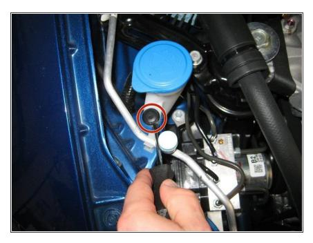
Pry up the center of the fastener with a flat-head screwdriver.
