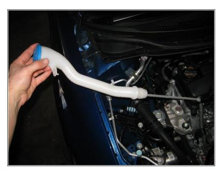
Remove the wiper fluid tube.
