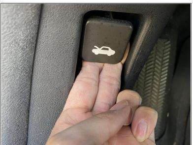
Lift the latch to open the car hood.
