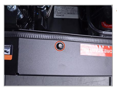
Use a 10 mm socket to remove the bolt securing the belt guard.
