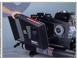
• Tilt the belt guard away from the device and lift it out to remove it.
