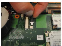
• Locate and remove the smaller white connector (far right) and any tape that is holding it down.
