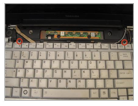
Remove the two 4mm flat-head screws indicated in the photo.
