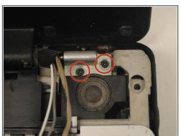
Remove the four 8mm button-head screws that are located in the top right (2) and top left corners
