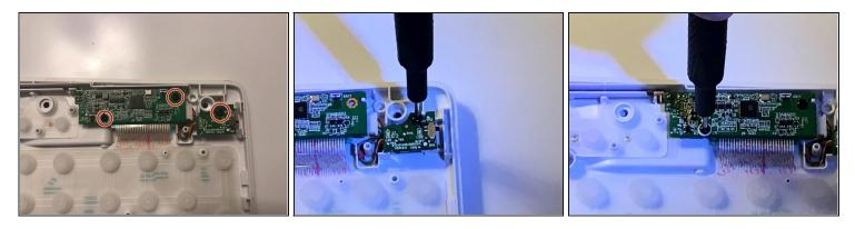
• Unscrew the circuit boards using a Phillips 000 screwdriver.
