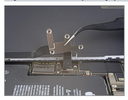
Remove the battery and display connector cover.
