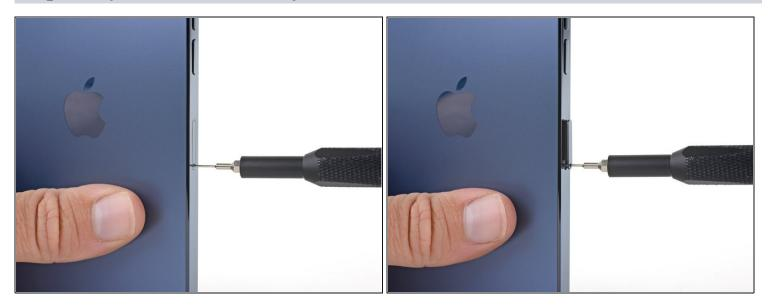
• Insert a SIM card eject tool or a paperclip into the small hole in the SIM card tray, located on the volume button edge of the iPhone.
