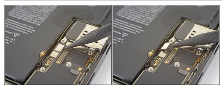
• Use the point of a spudger to pry the charging port connector straight up and out of its socket on the logic board.
