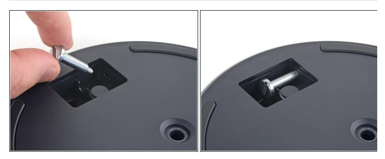
• Insert the screw into the cubby on the bottom of the stand.
