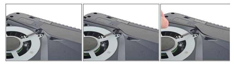
Insert the flat end of a spudger beneath the black wire cover and into the gap above the fan wires.
