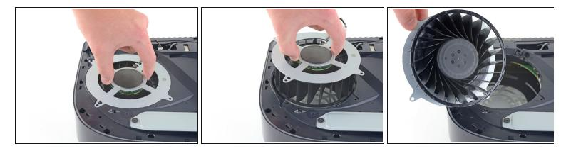
• Lift the fan up and out of the case to remove it.
