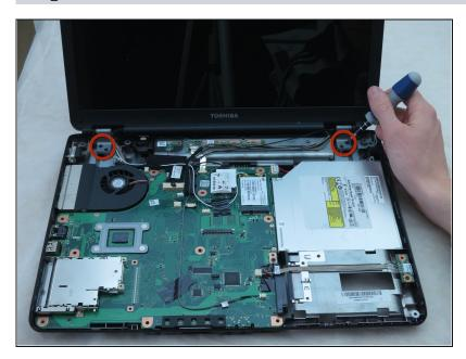
Remove the four 6-mm screws from the two hinge pads using a Phillips #1 screwdriver.
