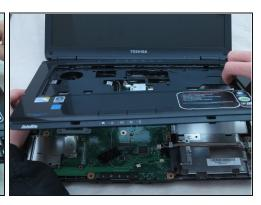
• Separate the laptop upper casing from the lower casing by using an opening tool around the sides of the case to pry it apart.
