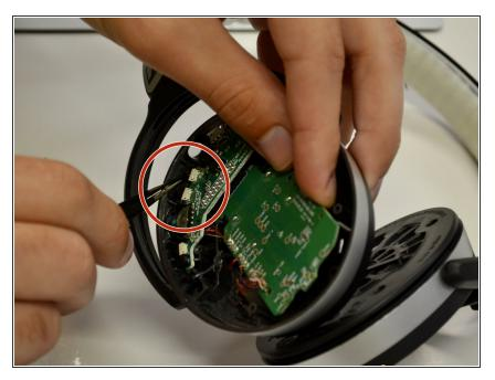
• Use a pair of tweezers to push the outer portion of the volume control button through the opening.
