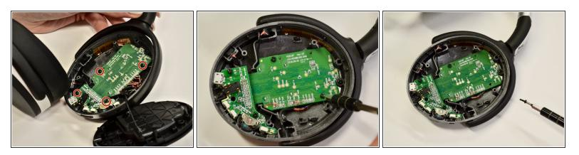
Use a Phillips #000 screwdriver to remove the four 6 mm screws holding the motherboard in place.
