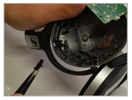
Using the tweezers, grasp the portion of the volume control button that is connected to the inside of the ear cup. Pull away until the button disconnects.
