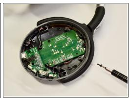
• Use a Phillips #000 screwdriver to remove the four 6 mm screws holding the motherboard in place.
