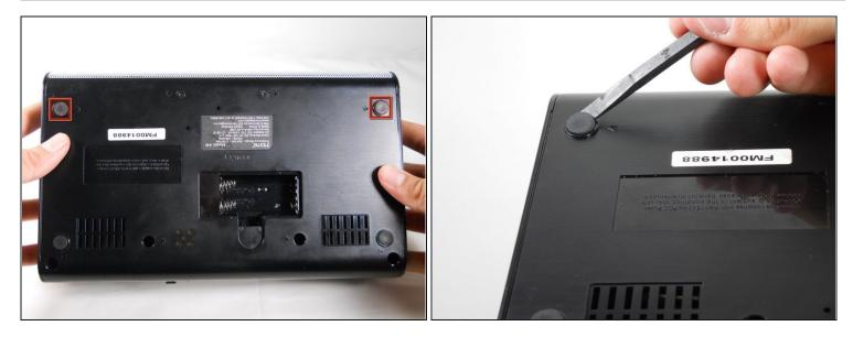
• Slide a spudger under the two front rubber pads to expose two hidden screws.
