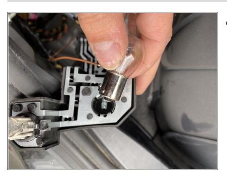
Pull out the bulb and repeat the process in reverse order with the new bulb to reassemble.
