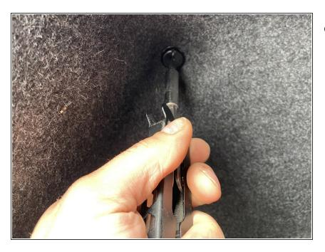
With a flathead screwdriver, turn the screws half a turn counterclockwise.
