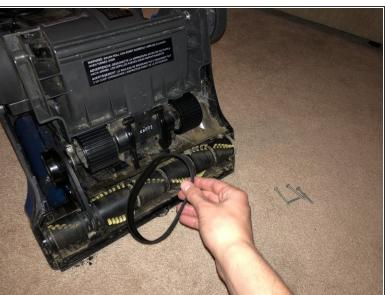
Remove the old vacuum belt by sliding the belt off the brush roller (the bottom roller), and then
