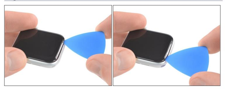
• Slide the opening pick around the corner to cut the remaining adhesive on the short edge farthest away from the crown.
