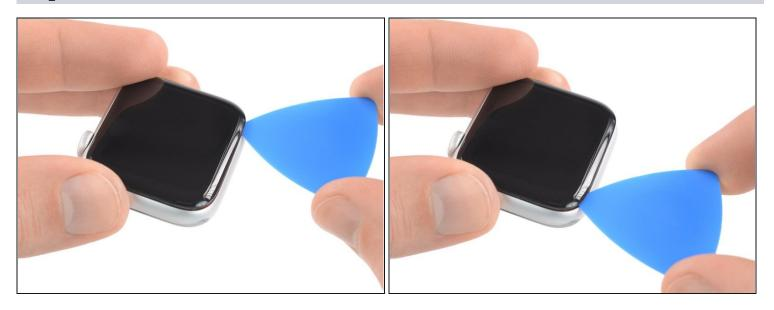
• Place the watch on a flat surface and use an opening pick to slice through any remaining adhesive.
