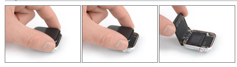
⚠ Be careful not to strain the display cables when you fold the display to the side.
