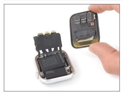
• Separate the watch assembly and the display.
