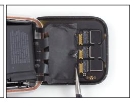
• Carefully pull the display flex cables out of their ZIF connectors.
