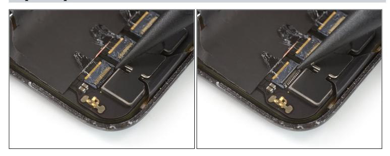
• Use the pointed end of a spudger to open the right ZIF connector on the rear side of the display by bringing its flap in an upright position.
