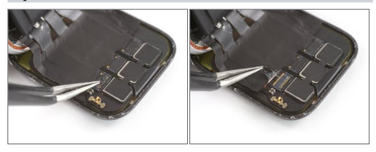
• Use a pair of <u>tweezers</u> to carefully peel off the tape covering the right display cable connector.
