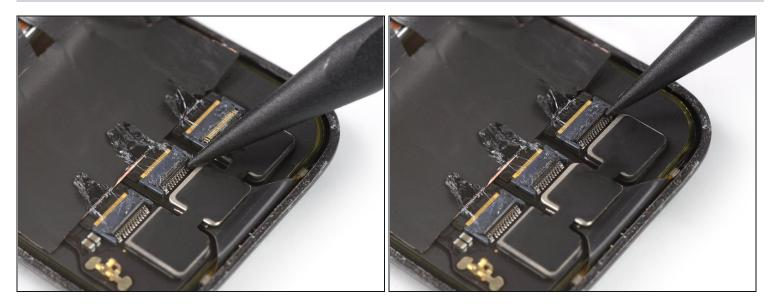
• Use the pointed end of a spudger to open the middle and left ZIF connectors by bringing their flaps to an upright position.
