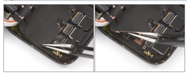
• Use a pair of tweezers to peel the right edge off the display cable sticker off the rear side of the display.
