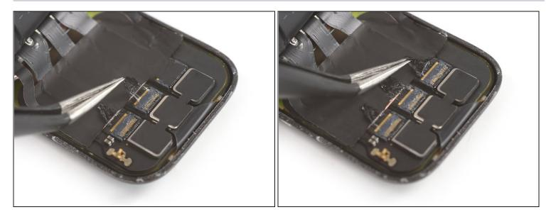
• Use a pair of tweezers to carefully peel off the tape covering the middle and left display cable connector.
