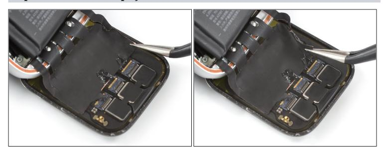
• Use a pair of tweezers to peel the left edge off the display cable sticker off the rear side of the display.
