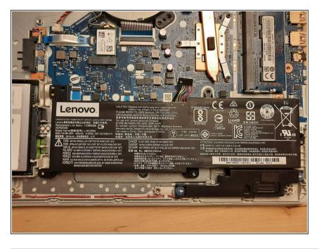
Lift the battery and place in the new one.
