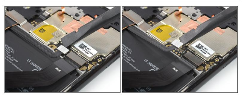
• Use the flat end of a spudger to pry up and disconnect the battery flex cable from the motherboard.
