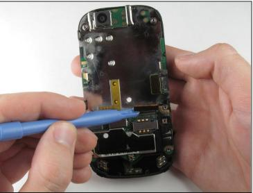
Pry the orange keyboard connector from its socket on the motherboard using the edge of the plastic opening tool.
