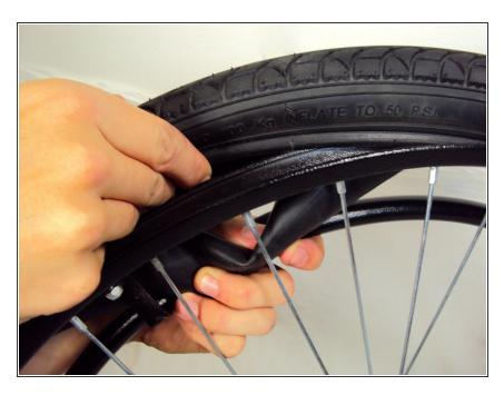
Reach inside the tire and remove the tube from the metal frame.
