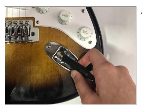
Test the tightness of your input jack before plugging your audio cable into your amplifier.
