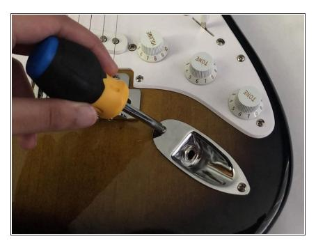
Carefully reconnect the plate back on using your screwdriver.
