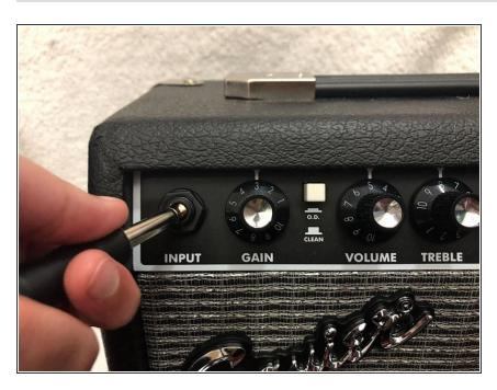
Plug the guitar into the amplifier to test the audio cable sensitivity and output quality.
