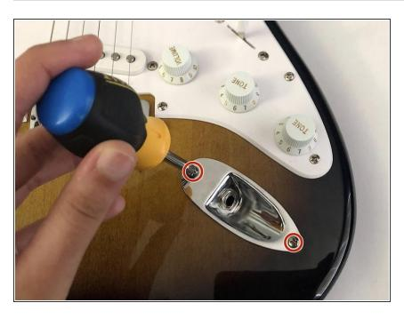
Using the Phillips #3 screwdriver, remove the two 1.2 mm screws that are connected to the plate.
