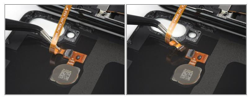
Disconnect the fingerprint flex cable by pulling it straight out off the ZIF connector using a pair of tweezers.
