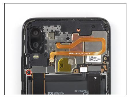
Use a Phillips screw driver to remove the 3.3 mm-long screw securing the display connector cover to the midframe.
