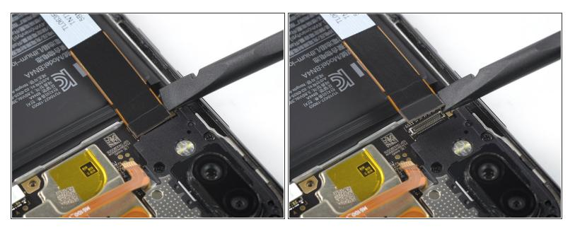
• Use the flat end of a spudger to pry up and disconnect the display flex cable.
