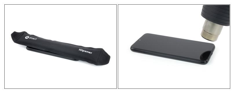
Apply a <u>heated iOpener</u> or a heat gun to the screen to loosen the adhesive underneath. Apply the iOpener for at least two minutes.
