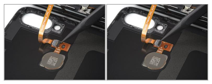
Use the pointed end of a spudger to open the ZIF connector by bringing its black flap in an upright position.
