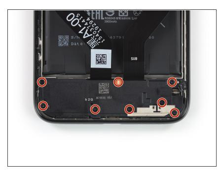
Use a Phillips screw driver to remove the eight 3.3 mm-long screws securing the loudspeaker assembly.
