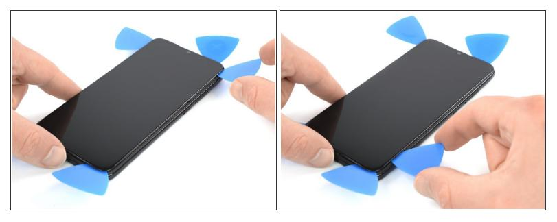
Insert a fifth opening pick and slide it along the right edge of the phone to cut the remaining adhesive.
