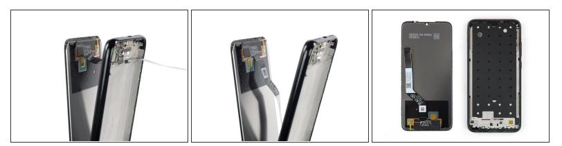
• Thread the display flex cable through the gap in the midframe and remove the screen.
