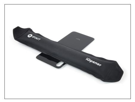
Heat an iOpener and apply it to the rear glass where the finger print sensor is located to soften the adhesive. Apply the iOpener for at least two minutes.
