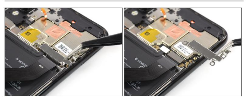
Use a pair of tweezers to remove the connector cover.
