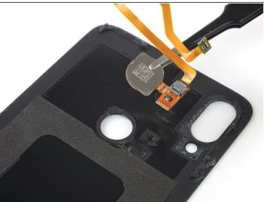
• Use a pair of tweezers to remove the fingerprint sensor assembly.
