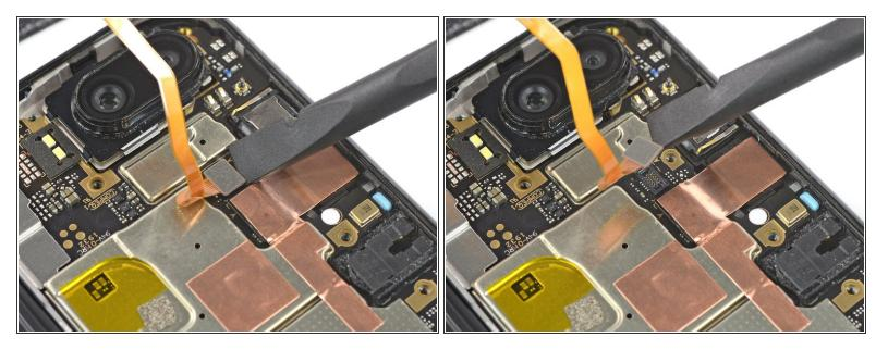
• Use the flat end of a spudger to pry up and disconnect the fingerprint sensor flex cable.
