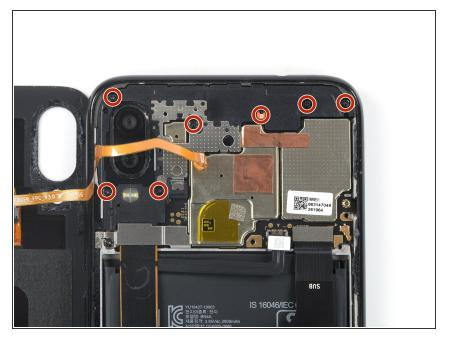
Use a Phillips screw driver to remove the seven 3.4 mm-long screws securing the motherboard cover.
