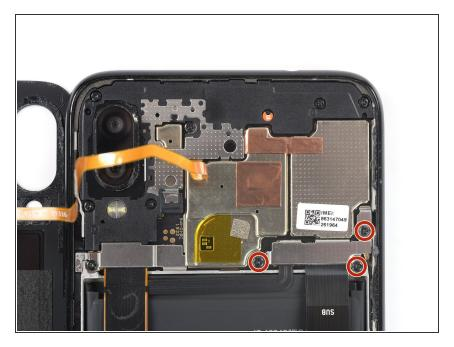
Use a Phillips screw driver to remove the three 3.3 mm-long screws securing the connector cover to the midframe.
