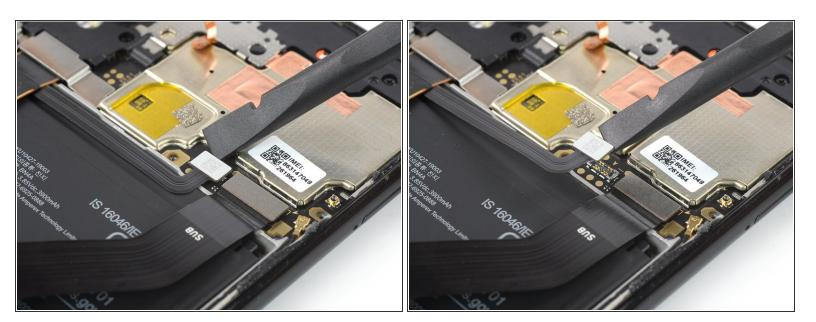
Use the flat end of a spudger to pry up and disconnect the battery flex cable from the motherboard.
