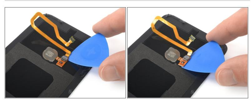
• Carefully slide an opening pick underneath the short orange flex cable with the ZIF connector on top to separate it from the rear glass.
