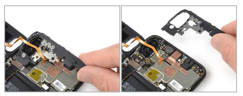
Remove the motherboard cover by pulling it in the direction of the top edge of the phone.
