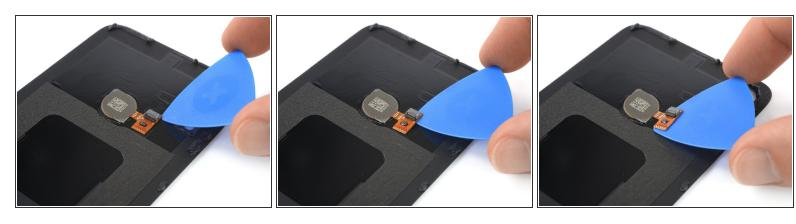
Carefully slide an opening pick underneath the orange flex cable with the ZIF connector to separate it from the rear glass.
