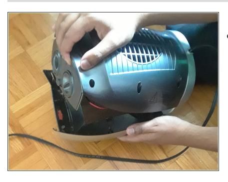
Separate the back case from the heater.
