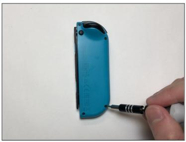
Use the Tri-point Y00 screwdriver to remove the four 6 mm screws from the back of the Joy-Con.
