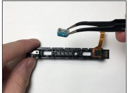
• Remove the SL, SR and sync buttons from the charging rail.
