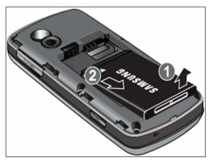
Gently lift up and remove battery with your fingers in the direction of the arrows.
