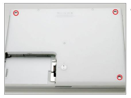
Remove the three newly-revealed Phillips screws.
